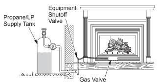
Figure 34 - Checking Gas Joints for Propane/LP Gas Fireplace
